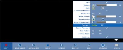
**b** Enable the Password function will pop up a character screen, key in a 4-digit number from the screen and press the **Enter** button.
