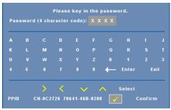
**CHANGE PASSWORD**—Key in the original password, then enter the new password and confirm the new password again.
